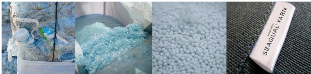
**Image 12.** Construction Stages of Seaqual Polyester Fibers and Fabric Sample (URL5, 2023).
