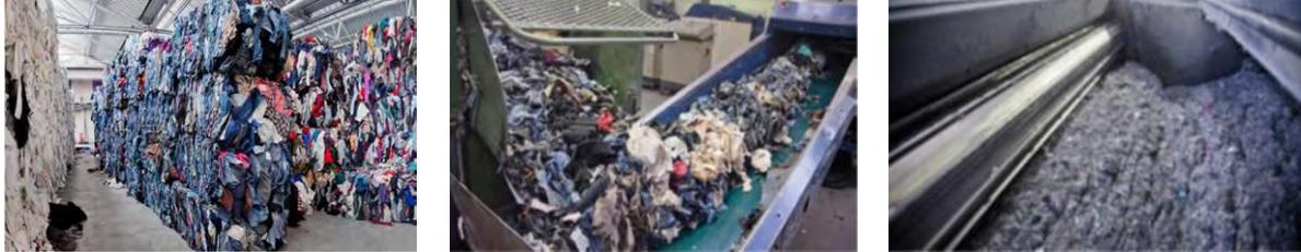
(a) Classification of Clothing Wastes (b) Shredding of Wastes in a Machine called Chiffonoz (c) Turning Wastes into Fiber
